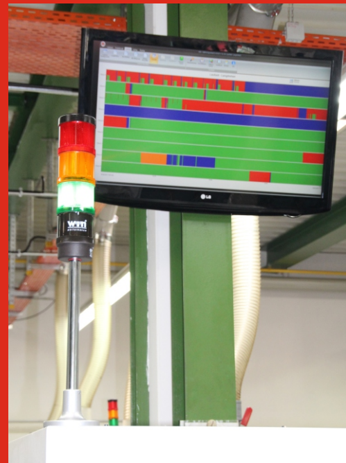
The software shows the status of the machines in the network and the client is able to analyse productivity, look at fault codes and then consider optimisation measures to improve the efficiency of the machine.
