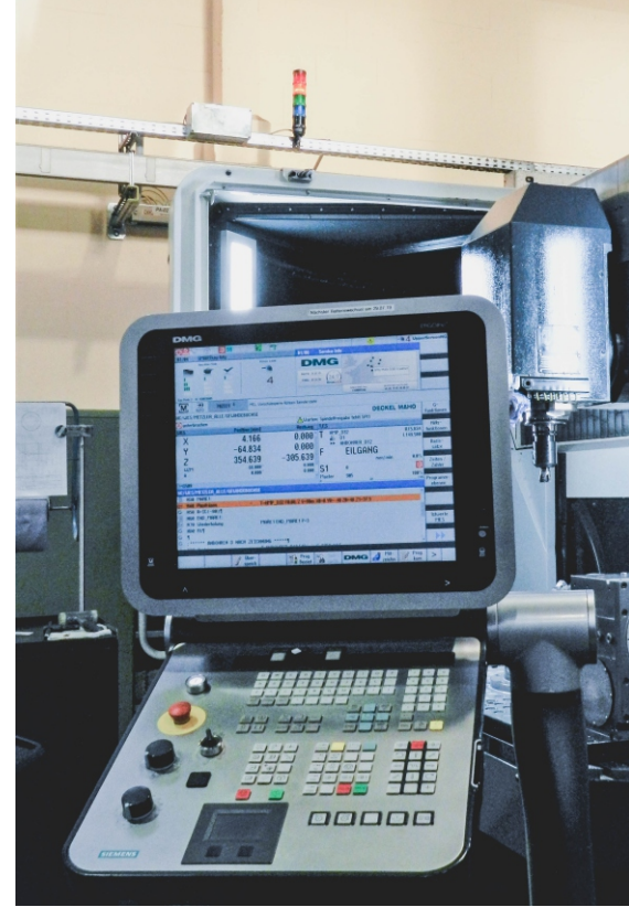
The signal towers were mounted above the machines and are also clearly visible from a distance
